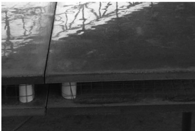
Fig. 11 The lightweight concrete panel has a sturdy clean, smooth, water-resistant surface
