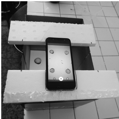
Fig. 6b EFSB feeding preference experiment setup using the camera of the mobile device
