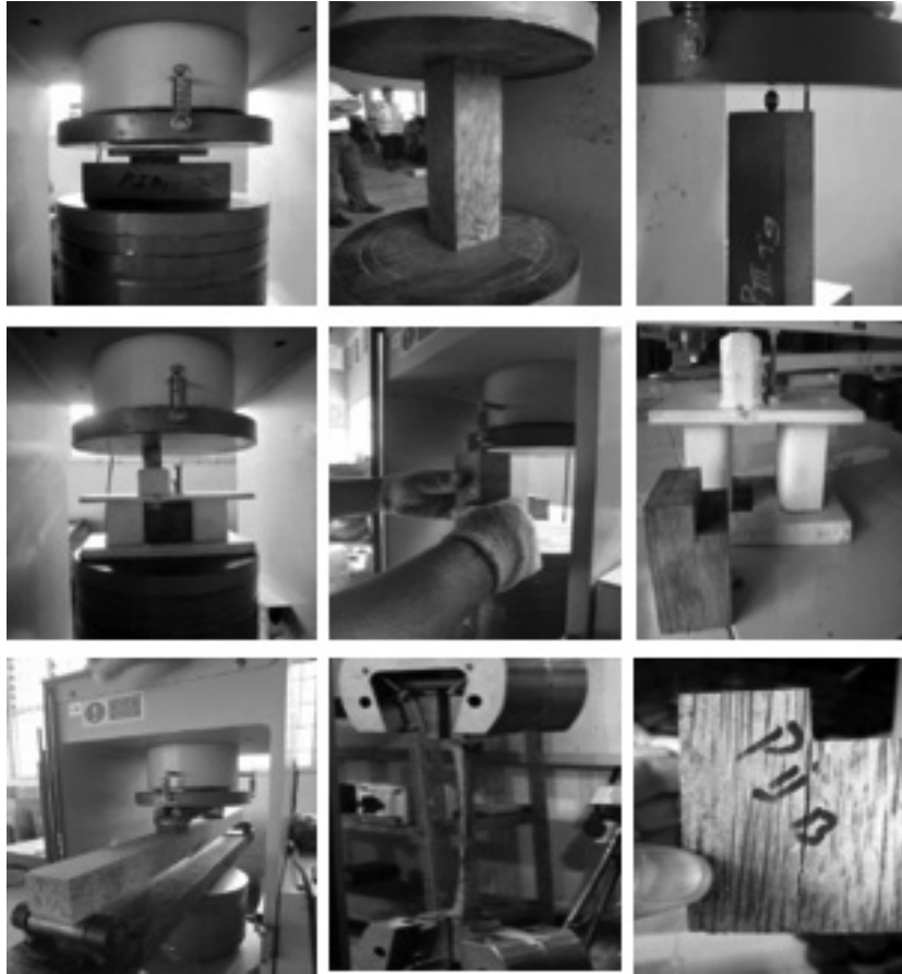
Fig. 2. Mechanical properties tests of coconut-timber at the Material Testing Laboratory, Manado State Polytechnic
