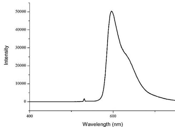
Fig. 3. Emission spectrum of FSNP at excitation wavelength  $553 \text{ nm}$
